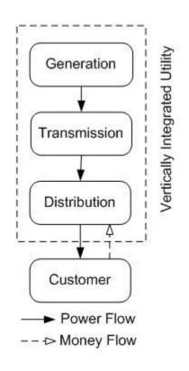
The term "vertically integrated utility" refers to a utility that owns all levels of the supply chain: generation, transmission, and distribution.
